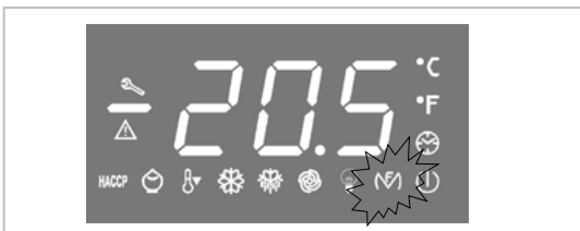
This LED indicates the state (on or off) of the DOOR RESISTANCES
