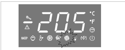
This LED indicates the state (on or off) of the FAN
