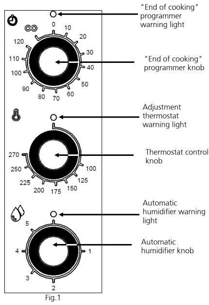
**Programming cooking time** - The oven is switched on by turning the programmer knob (Fig.1) to the **U** symbol (continuous operation) or to the selected cooking time (up to 120 minutes); in the latter case the end of cooking is signalled by the oven switching off automatically.
